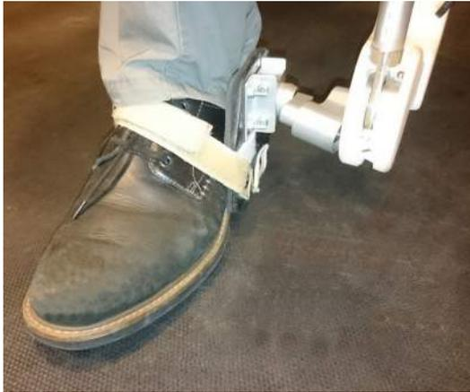
(c) Detail on the second foot bracket and its interface with the ankle gimbal.
